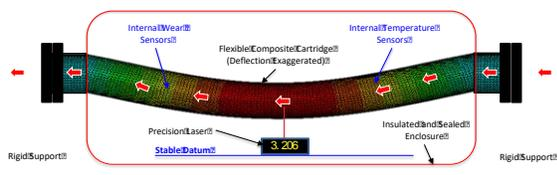
Figure 1: Basic Operating Concept – Critical Components
