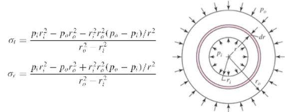
Figure 2: Relationship of Pressure and Stress
