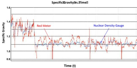
**Figure 4: Red Meter vs. Nuclear Density Meter**
