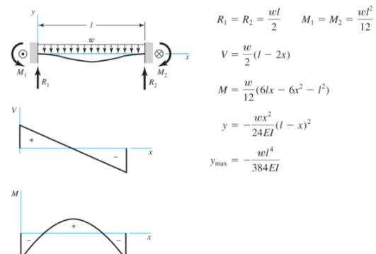
Figure 3: Relationship of Load and Beam Deflection
