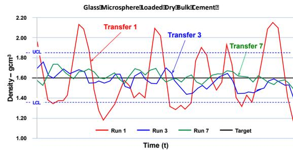
Figure 7: Dry Bulk Blend Identification
