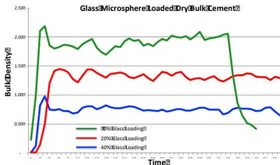
Figure 6: Dry Bulk Blend Identification
