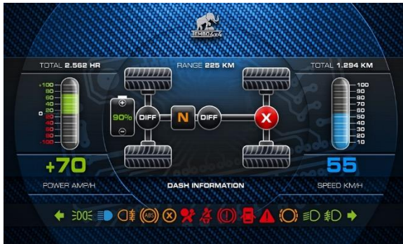
The digital instrument cluster enhances the Tembo 4x4 e-LV operator experience.
