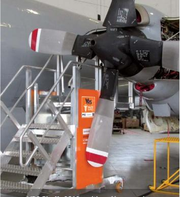
VRS Giraffe 2310 positioned by an engine of a 5 Squadron RNZAF P-3K2 Orion aircraft undergoing maintenance
