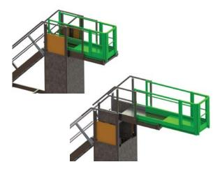
The slide out cantilever is a semi-permanent, factory mounted option that can simply and effortlessly be rolled out at any time (while the user remains within the safe confines of the deck) to achieve a massive 1400mm extra extension. (Reduced load capacity applies)
