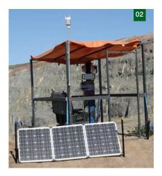
Inspections indicated that block toppling might eventuate so alarms were set in the Sentry system at 2mm/ hr (geotechnical alarm) and 3mm/hr (critical alarm).
