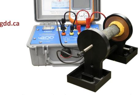
Get the information that you need to design an appropriate geophysical survey! **SCIP** is an innovative way to measure electrical properties of drill cores, hand samples or outcrops. Provides real time feedback. Relates DDH cores to resistivity and IP survey results. Allows constraining geophysical inversions.
