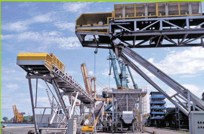
Mobile ship unloading system with loading hopper and belt conveyor system
