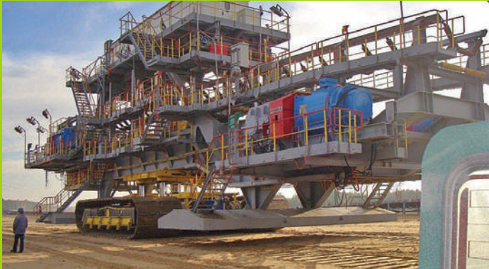
Drive station B=2250 mm, 4x1250 kW with PIOMA drive units
