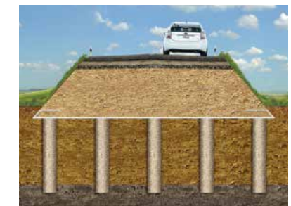
Geotextile Encased Columns (GEC)
