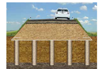
Geotextile Encased Columns
