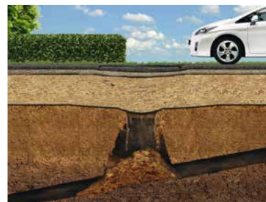
Bridging of Sinkholes
