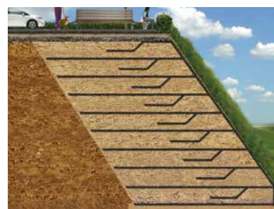
Geosynthetic Reinforced Soil
