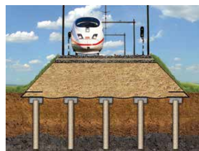
Embankments on Piles
