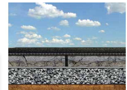
Rehabilitation of Concrete Pavements with Asphalt
