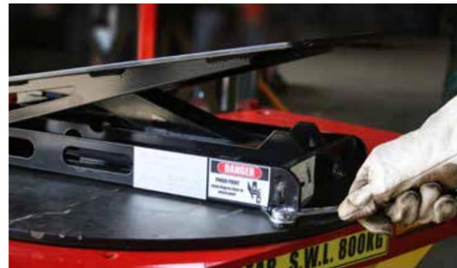
Table top attachments mount quickly and securely to the turntable with 4 x M12 bolts. The rotating turntable provides ease of movement when lining up components and bolt holes. (Pictured Above)
