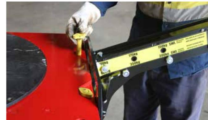
Changing front attachments can be done in moments; simply pull out the two yellow attachment pins, remove the existing attachment, slide the chosen attachment eyelets into the frame and replace the pins. (Pictured Above)
