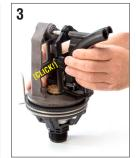
Reinstall plate assembly. Guide shift lever between stops as shown in Fig. 4.
