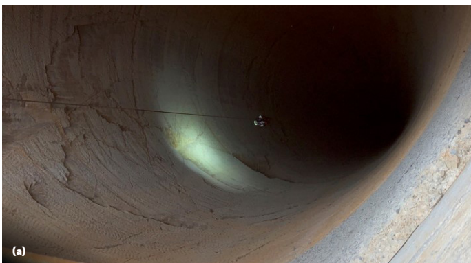
a) Lowering Hovermap down a raisebore shaft, 5m diameter, 500m depth, by cable and the (b) resulting point cloud obtained.
