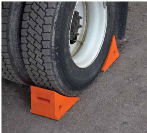
Checkers urethane chocks model UC1500 used on a utility truck
