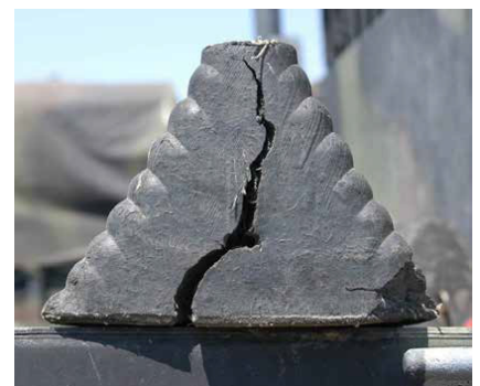
Rubber chocks are more susceptible to cracking and breaking
