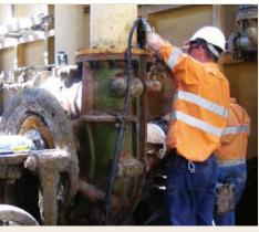
EQUIPMENT EXAMPLE: A slurry pump transporting tailing experiences wear at the suction throat, backplate, impeller, and cutwater. Wear at these critical tolerance areas impacts pump performance and efficiency, requiring longer operational cycles to meet plant demand.
