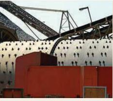
EQUIPMENT EXAMPLE: A SAG mill experiences wear of mill media and mill liner during grinding phase. Mill media wear reduces grinding effectiveness in the mill and increases the reject rate at the mill discharge/ hydrocyclone.
