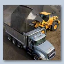
**Volvo L250G Rehandler** is designed specifically for **two pass loading** of finished aggregate product in triaxle onhighway trucks for up to 30% more trucks loaded per day.
