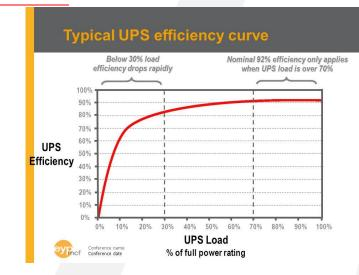
At idle (unloaded), all the energy drawn by a UPS is lost as heat, noise or earth leakage. For example, a 20kW UPS, unloaded, may draw 800 Watts of power, while out putting zero watts. That's not particularly efficient. The efficiency comes in when the UPS is running at something like 75% load, where it's putting out 17.5kW of energy, and is probably only dumping 1800 watts of waste energy as heat and noise.
