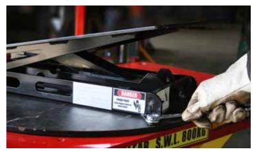
Table top attachments mount guickly and securely to the turntable with 4 x M12 bolts. The rotating turntable provides ease of movement when lining up components and bolt holes. (Pictured Above)
