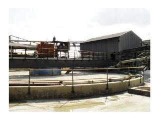
Another example of this is the refurbishment of two (2) 45.7m diameter thickener mechanisms for a gold operation. Thickeners that have been dormant for years can now be put back in operation for minimal investment. This enables the mining operation to increase production thus producing more products (gold in this instance) and stays economically viable.
