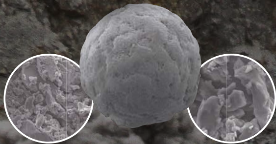
Electron Microscopy of Prillex® LR crystallization and whole Prill grain.
