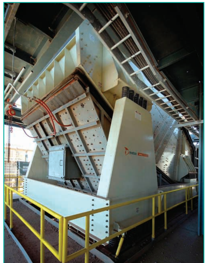
3.6 m x 8.2 m DD secondary Multi-Flo screening -7" material at up to 4,000 tph at copper mine in North America
