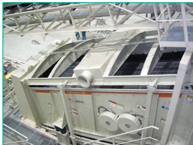
Screen matched with Trellex media and dust enclosure
