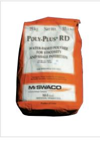
POLY-PLUS\* RD acrylic copolymer (PHPA) is a readily dispersible product designed to provide cuttings encapsulation and shale stabilization. It is formulated for easy mixing with improved dispersion to eliminate "fish eyes." This is beneficial when rapidly mixing either large quantities or high concentrations of polymer where good mixing equipment is unavailable. POLY-PLUS RD acrylic copolymer acts as a viscosifier, friction reducer and flocculant. It also provides some fluidloss control.
