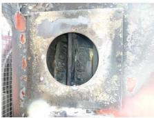
Figure 1: Severe slipring flash over
