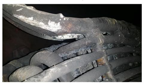
Figure 4: Consequence of re-switching on to the fault identified above
