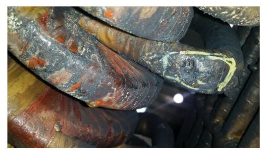
Figure 3: Fault at stator winding series connection
