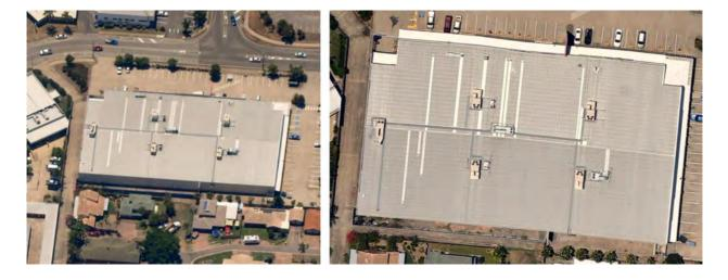
The site itself appears to be a large low pitched roof, with aged (& stained) zincalume steel sheeting. The roof area is approximately 3,900m<sup>2</sup> & would absorb extreme solar radiation exposure.
