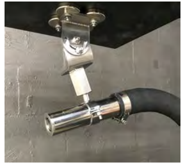
Plumb the cool air to an "Adjustable Magnetic Remote Silencer Mount"
