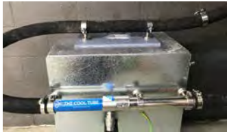
Plumb the cool air to an "Adjustable Magnetic Remote Silencer Mount"
