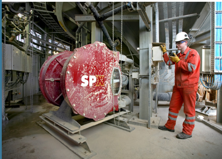
Bredel SPX pumps such as this one at Buxton Lime in the UK, have a corrosion-resistant enclosure which suits arduous mining environments.
