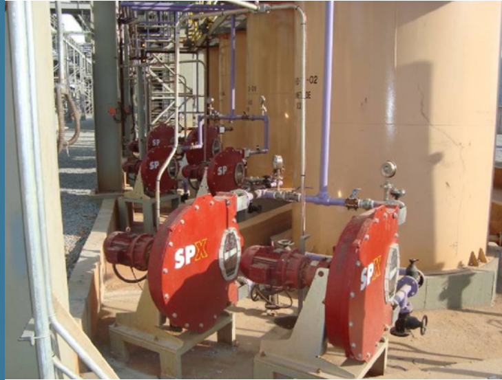
Bredel SPX65 on reagent dosing at Jaguar Mining, Brazil.
