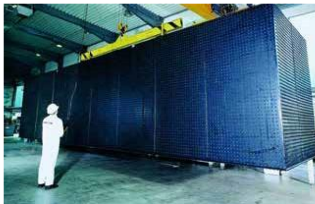
Above picture: A hydrochloric acid pickling plant is renovated using a pre-fabricated Bekaplast™ immersion tank accommodating contents of over 100 m³ thereby saving lots of time.
