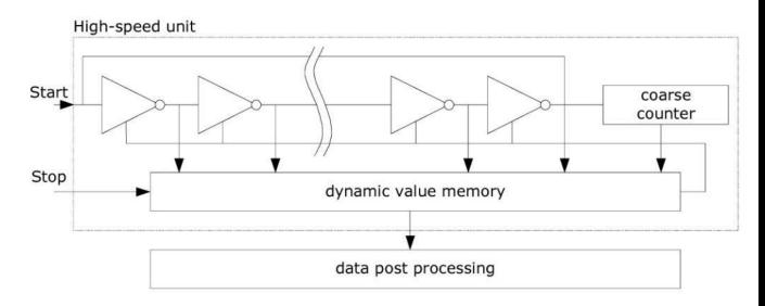
An output pulse is generated by the high speed field programmable gate array device which is injected into the cable. After a precise "guard time interval" the Time to Digital Converter is supplied with a start pulse. The detector circuit then produces a "stop" pulse when the original injected pulse is reflected from either an open or short circuit back to the unit. This "stop pulse" halts the Time to Digital Converter and the time elapsed is saved.
