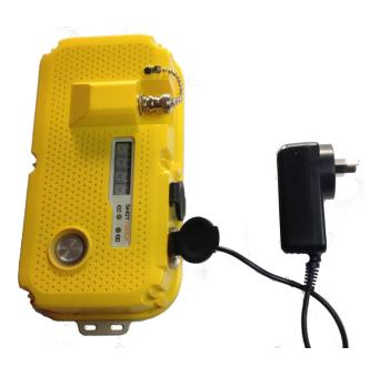
Charging is accomplished by plugging a standard 12-volt plug pack into the right hand rear socket.
